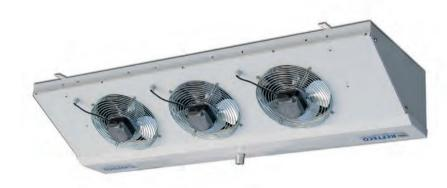
Angled air coolers super compact for small storage cold rooms with volume from 10 to 50 m3. Thanks their heavy metal construction they are suitable for storage of fresh or frozen food with temperature from -25 to +20°C.
