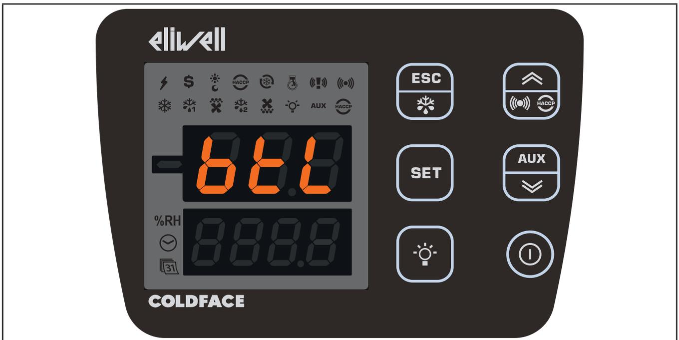
**RCN●●●●●●●●●●** models: when the HACCP Module is connected and the Bluetooth connection to the Eliwell Air App is active, the btL label appears on the TOP DISPLAY and the BOTTOM DISPLAY and icons are turned off.
