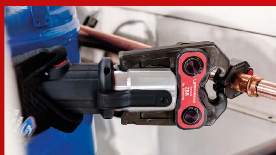
The 180° swivel allows a freely adjustable positioning of the press machine
