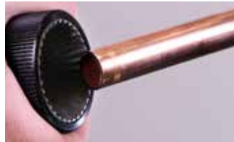
2. Deburr and remove all external sharp edges
