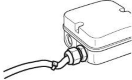
Fig. 2: Fan installed lying flat, cable routed in a U-shaped loop.
