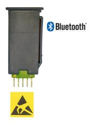
Attention, electrostatically sensitive components! Note chapter mounting the module.
