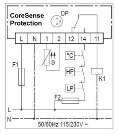
Figure 20: Control circuit wiring diagram
