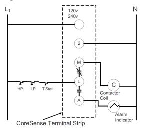
Figure 24: CoreSense module wiring diagram
