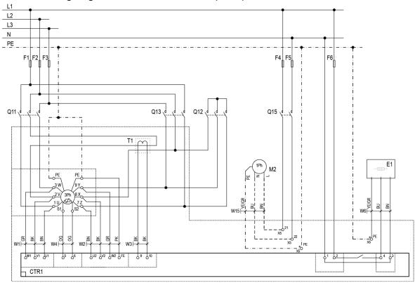
Figure 11: Wiring diagram - Star / Delta motors (EW...)
