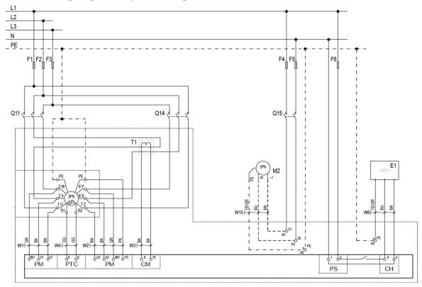
Figure 10: Wiring diagram – Part-winding motors (AW...)
