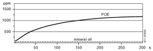
Figure 27: Absorption of moisture in ester oil in comparison to mineral oil in ppm by weight at 25 °C and 50% relative humidity (h=hours)
