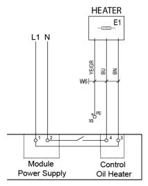
Figure 26: Heater connection diagram
