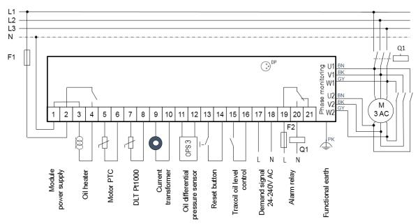
Figure 9: Basic module connections
