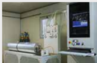
Permeability machine To evaluate the permeability of GOMAX QUADRA hoses for every batch according to EN 1736
