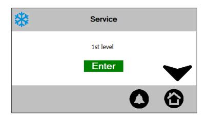
Press  $\checkmark$  button can switch to higher user level. For 2<sup>nd</sup> and 3<sup>rd</sup> level, relevant password is required.
