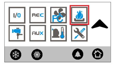
In auxiliary heating screen, set points and output status are displayed.
